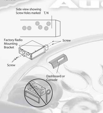
To fasten the unit to the factory radio mounting brackets.
